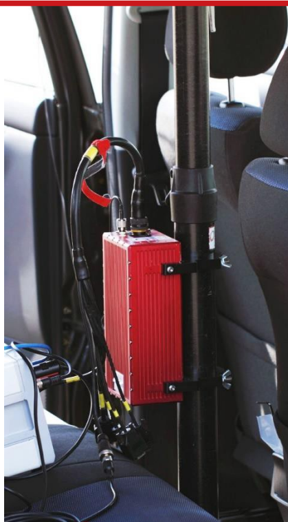
Figure 18. An RT device mounted on our RT-Strut
